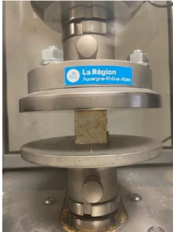
Figure 12: bending test (left) and compression test (right)
