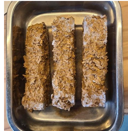
Figure 13: problem of demoulding and bricks malformed
