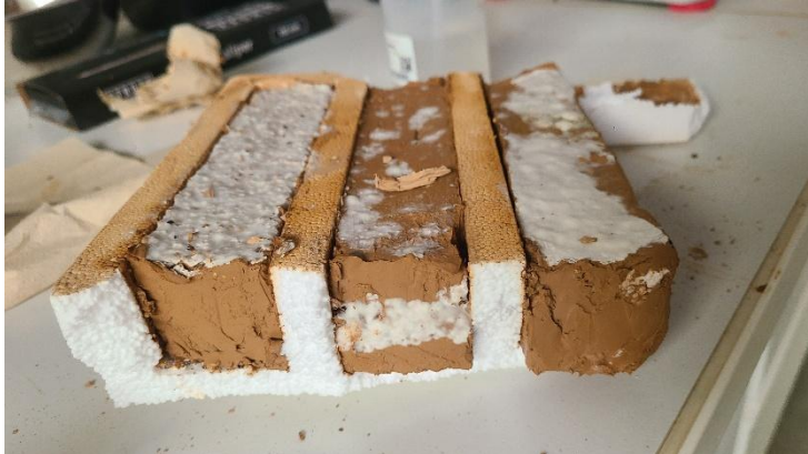
Figure 24: mycelium development on different layers
