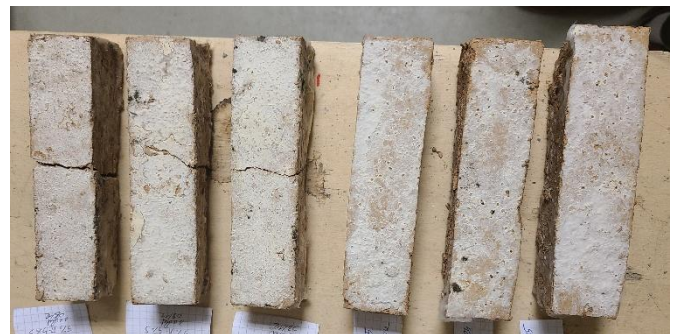
Figure 18: difference between brick with and without sugar
