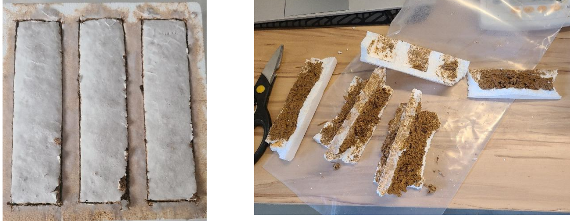
Figure 9 : A cut-out with a cutter (left), a poor demoulding (right)
