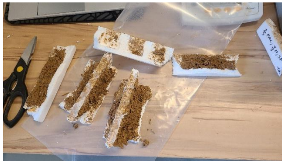
Figure 13: problem of demoulding and bricks malformed
