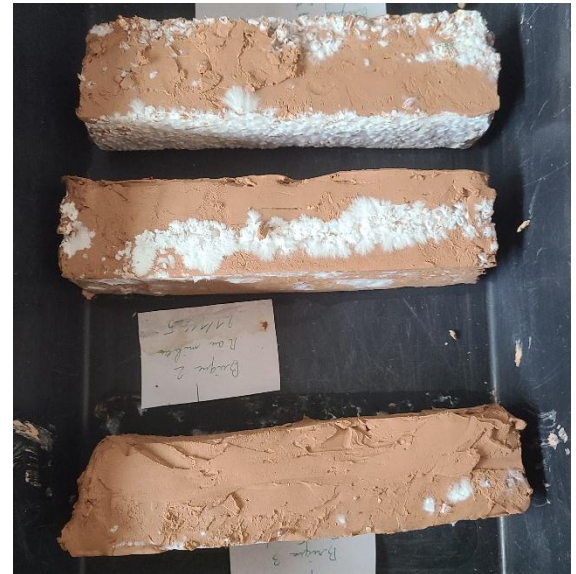
Figure 24: mycelium development on different layers
