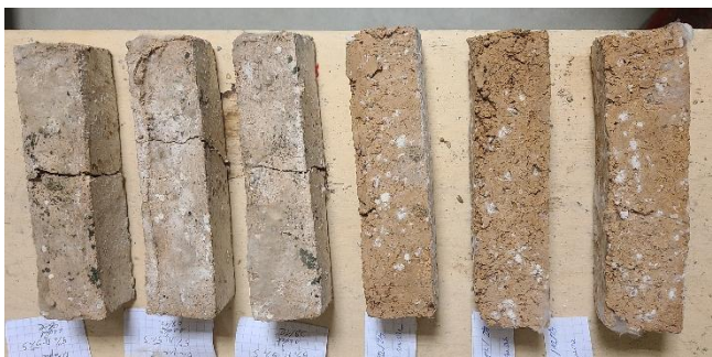
Figure 18: difference between brick with and without sugar
