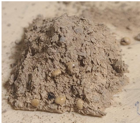
Figure 26: pyramid remaining after compression test
