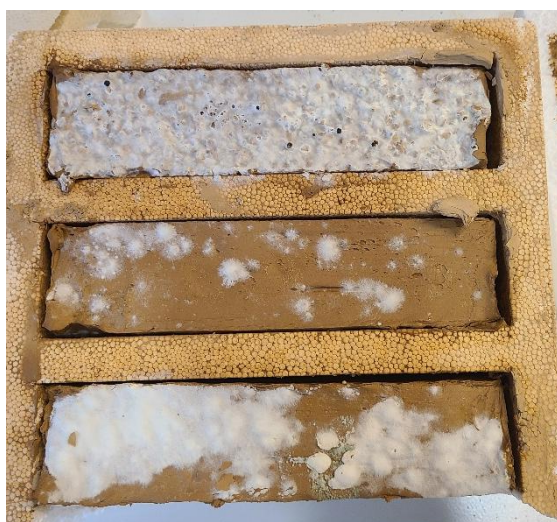
Figure 23: bricks with mycelium at different level
