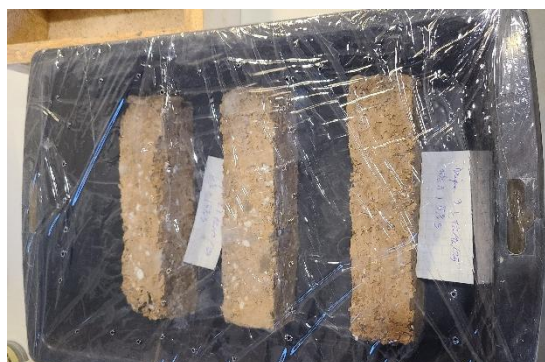
Figure 10 : bricks in plastic basin covered by a film for the surfacing
