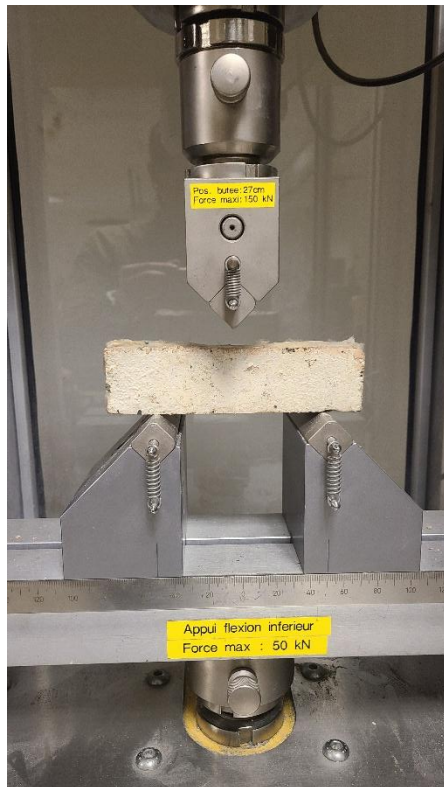
Figure 12: bending test (left) and compression test (right)
