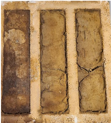
Figure 21 : control bricks with 100% FAC+ sugar (the 2 bricks on the right) + sawdust (brick on the left)
