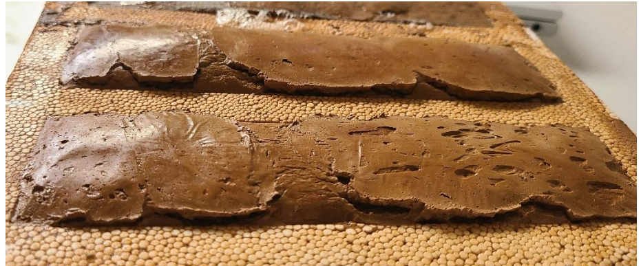
Figure 21 : control bricks with 100% FAC+ sugar (the 2 bricks on the right) + sawdust (brick on the left)
